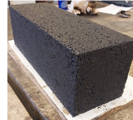
Slab prepared using IPC Global Pressbox slab compactor
