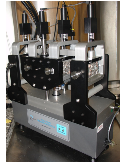
Specimen setup in four-point flexural fatigue test device
