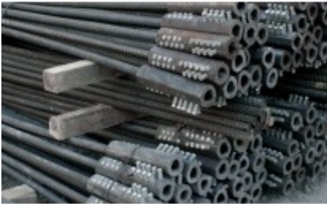
A1035 rebar can be threaded and can be turned into headed terminator
