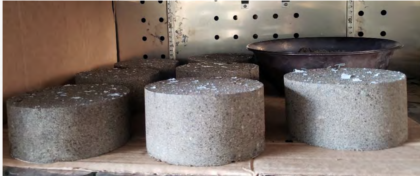
FDR at 1% cement, 3% Emulsion and 3% water (Mix B)
