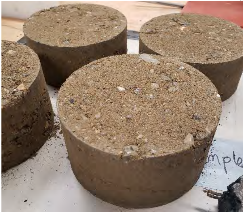
FDR at 4% cement and 3% water (Mix A)
