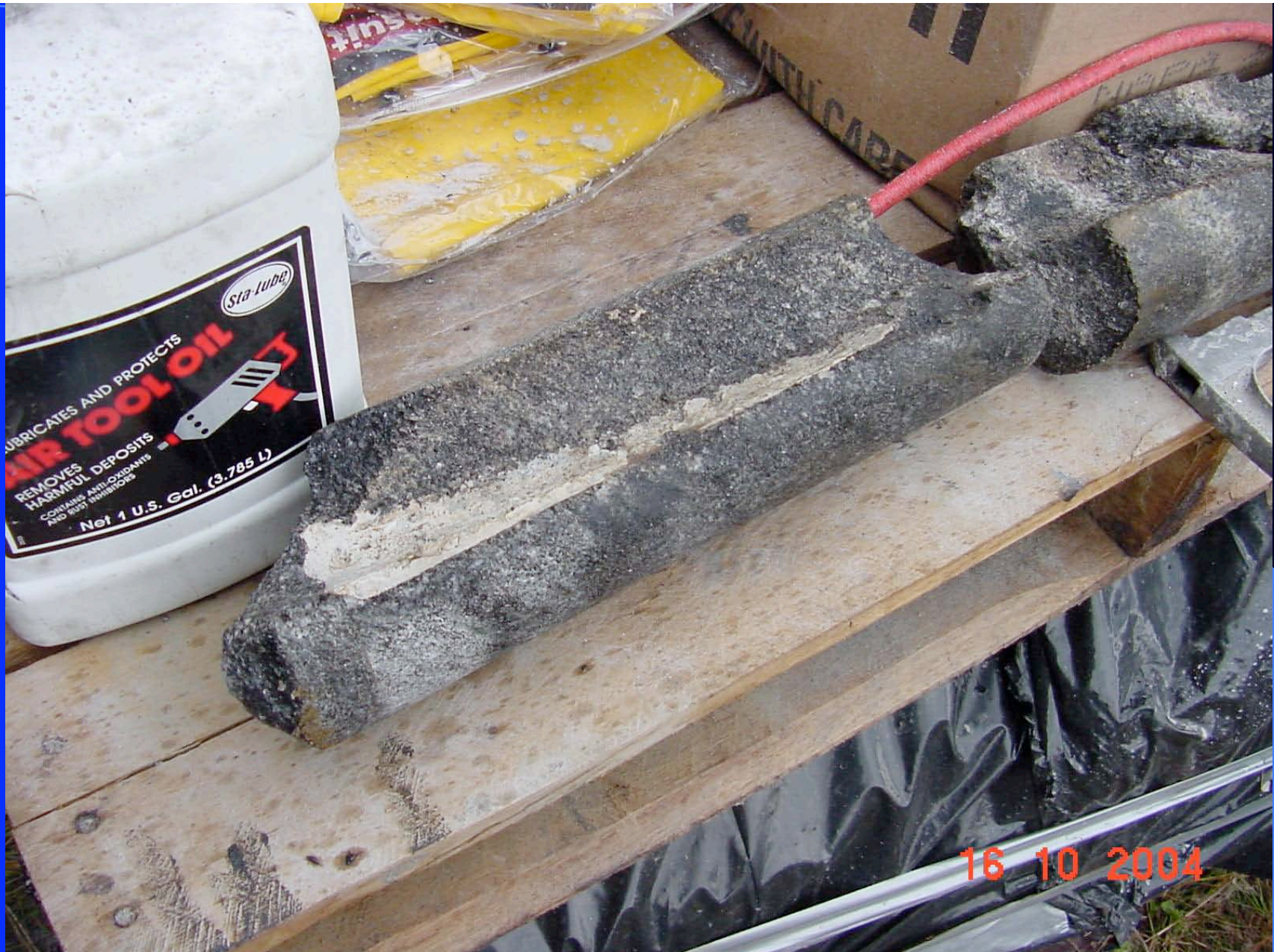
Recovered Resin Grout
