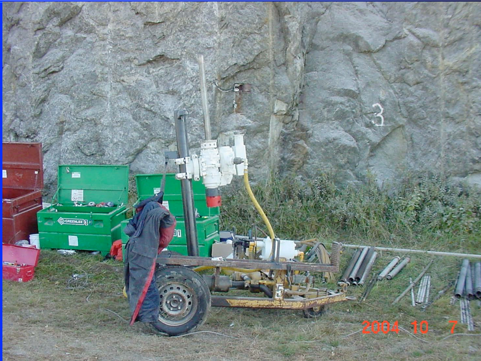
Drill Rig for Over-coring Rock Reinforcement
