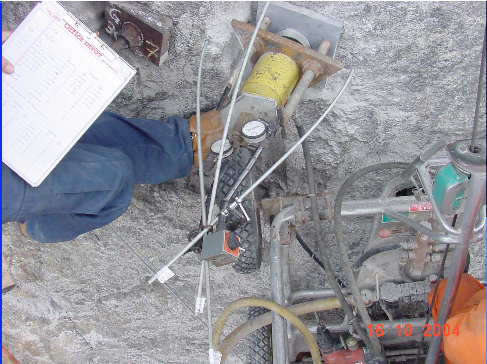
Proof Test on New Rock Bolts
