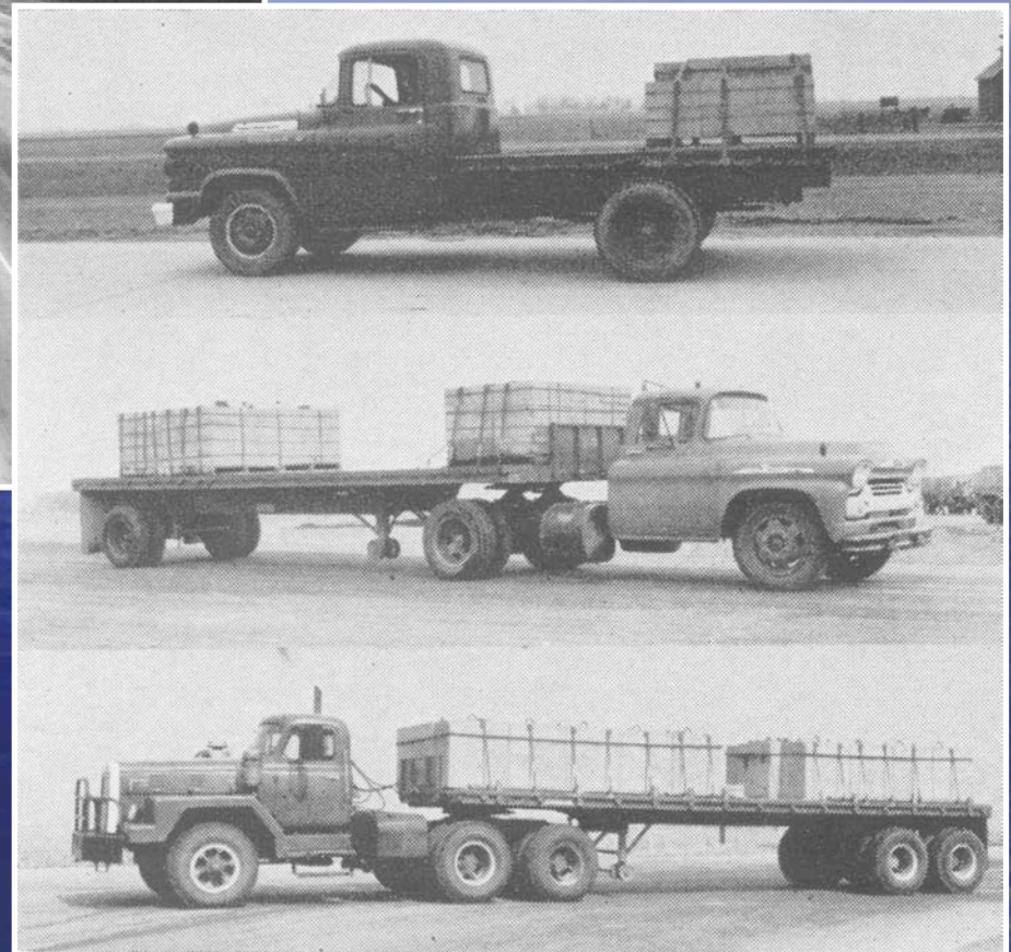
Figure 23. Test vehicles, showing typical axle arrangements and loadings.
