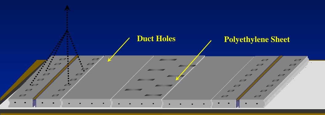
Joint Panel Base Panel C.S. Panel Base Panel Joint Panel (Multiple) Traffic Flow
