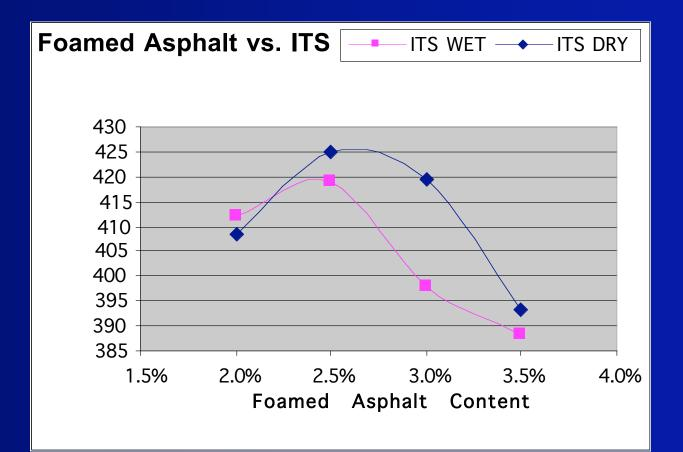
Foamed Asphalt vs. ITS Retained
