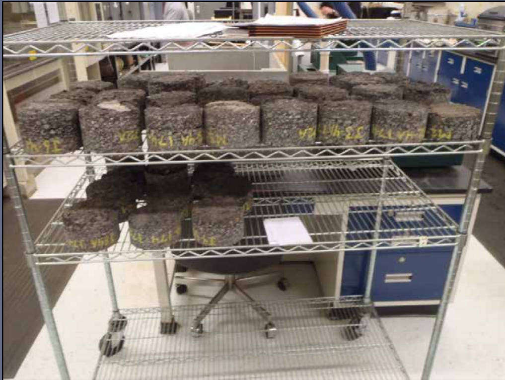
Secured cores ready for testing
