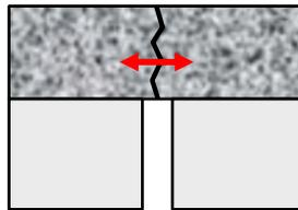
Mode 3: Horizontal Tensile Stress due to climate
