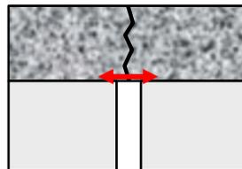
Mode 2: Horizontal Tensile Stress due to load
