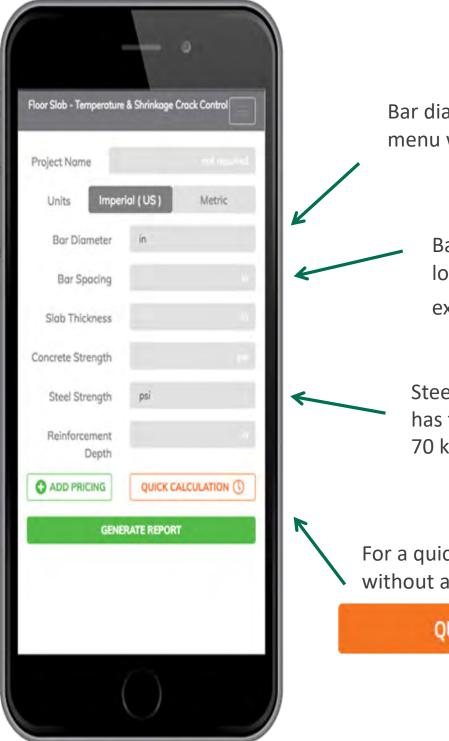
Bar diameter has a "drop down" menu with common options for size
