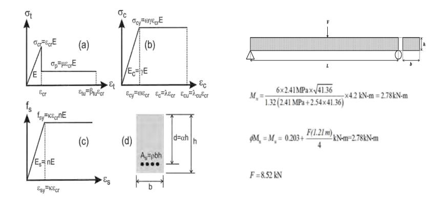
Material model for singly reinforced concrete design
