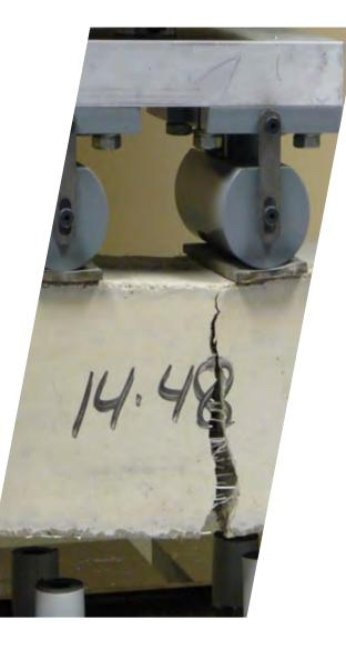
Crack control (bridging) in FRC beam under flexural loading
