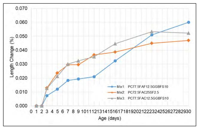
Alkali-silica reaction test results.
