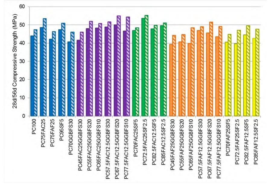
Mortar average compressive strength results for 28 day (solid bars) and 56 day (hatched bars) strength for mixtures tested.
