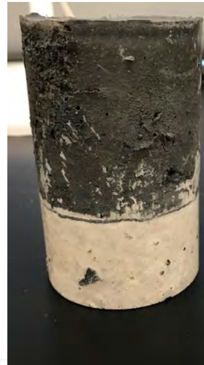
Composite cylinder (HPC and UHPC)
