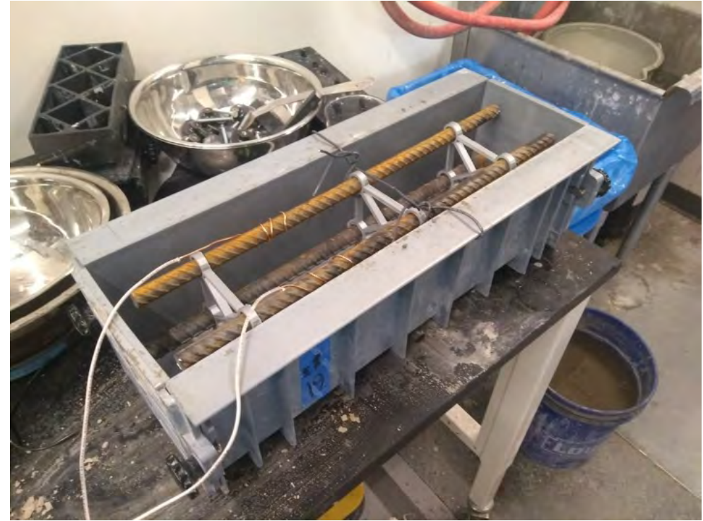
Beam for Top corrosion
