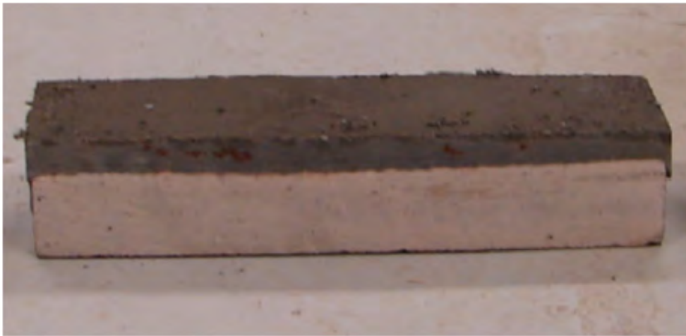
6 in. x 6 in. x 21 in. composite beam ( 4 inch of HPC and 2 inch of UHPC)
