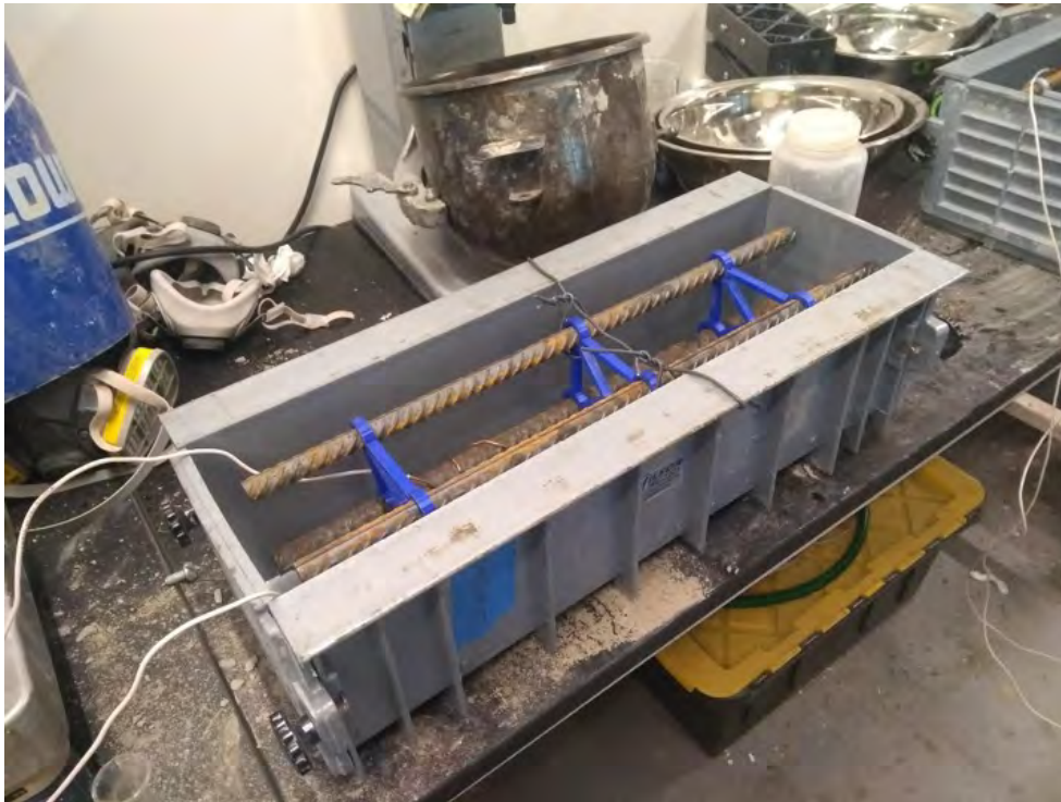
Beam for Bottom Corrosion
