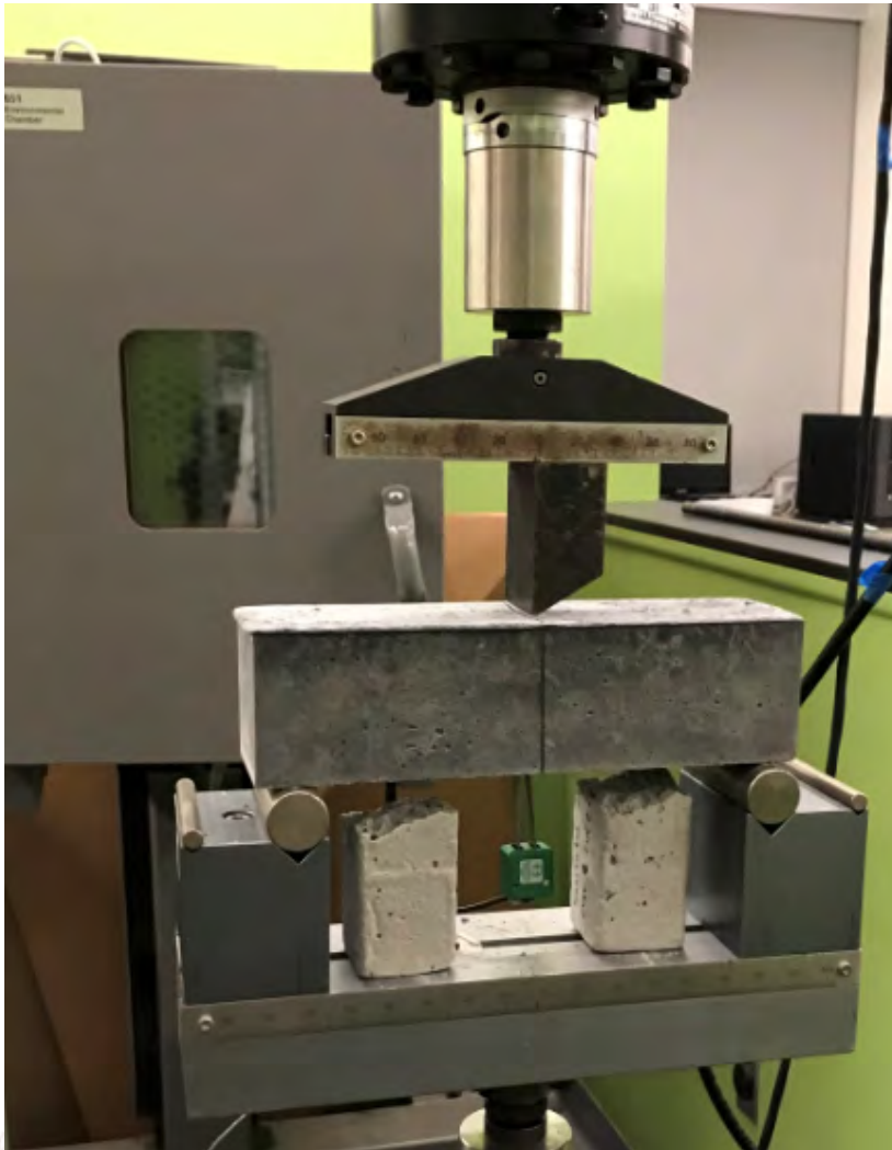
Experimental Set up of No Notch UHPC Beam
