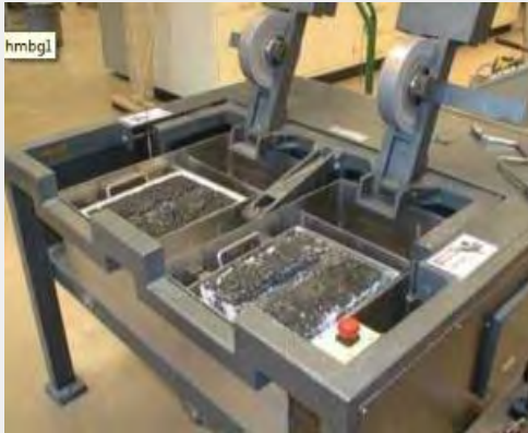
Hamburg Wheel Test (HWT)
