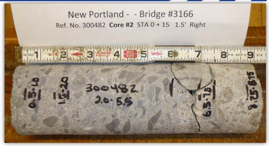
Concrete cores pulverized and analyzed for chloride content ~ rebar corrosion begins at 1.35lb/cy or 0.03%
