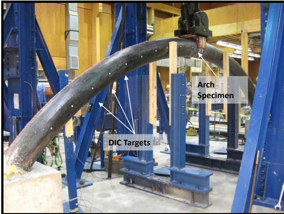
*Static & fatigue testing of over 40 specimens*
