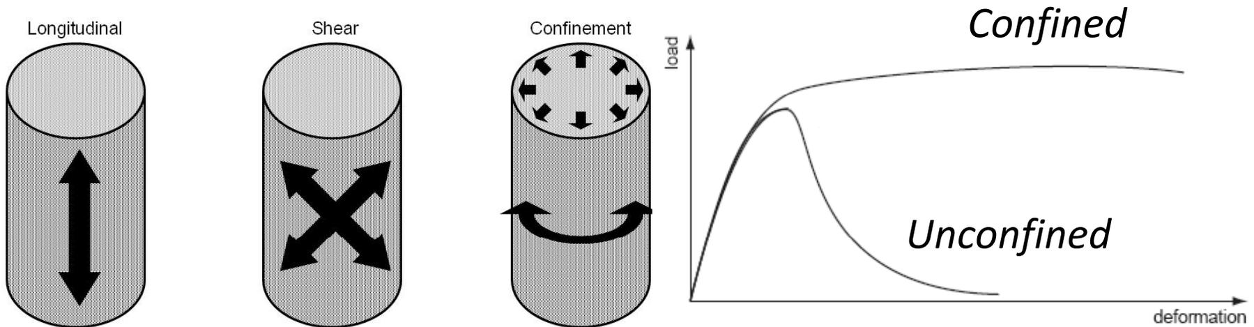
Three Components of FRP Reinforcement
